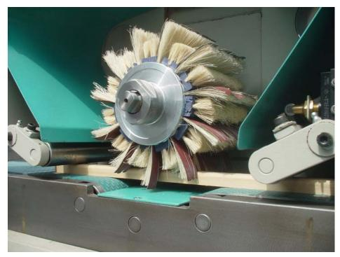
The optional **"GapSystem"** forces the belt away from the brush. When sanding thin work pieces, it is possible to set the brush down very deeply without touching the feed belt
