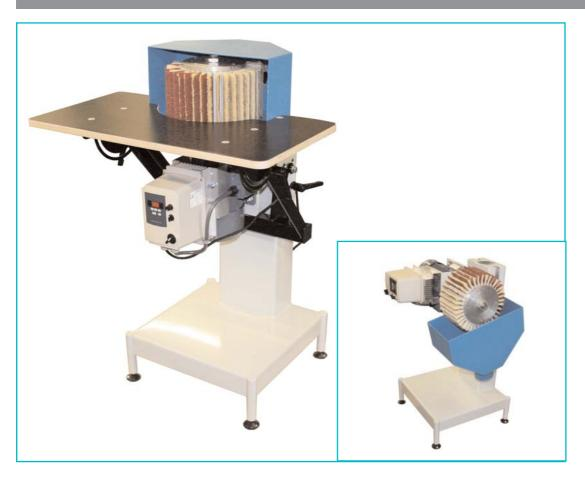
The LOEWER MiniSpin V is designed for whitewood sanding and lacquer / sealer sanding of profiled and non-profiled edges. The work piece will be moved manually along the rotating brush sanding unit.
