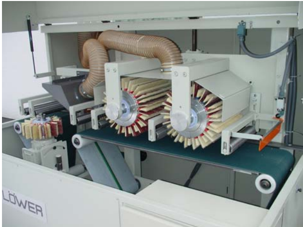
The inside of an LZ 3D with belt feed and hold down rollers shown left. Side heads shown right.
