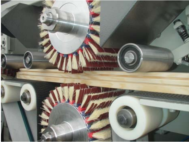
The inside of an LZ 4 with top and bottom heads and hold down rollers shown left. Side heads shown right.
